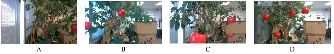
Fig. 7. The four scenarios labeled A , B , C and D used to assess the position accuracy obtained with the eye-in-hand RGB-D camera.
