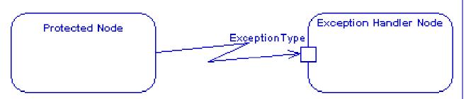
Exception handlers can be modeled on activity diagrams through the use of an **interrupt flow**
