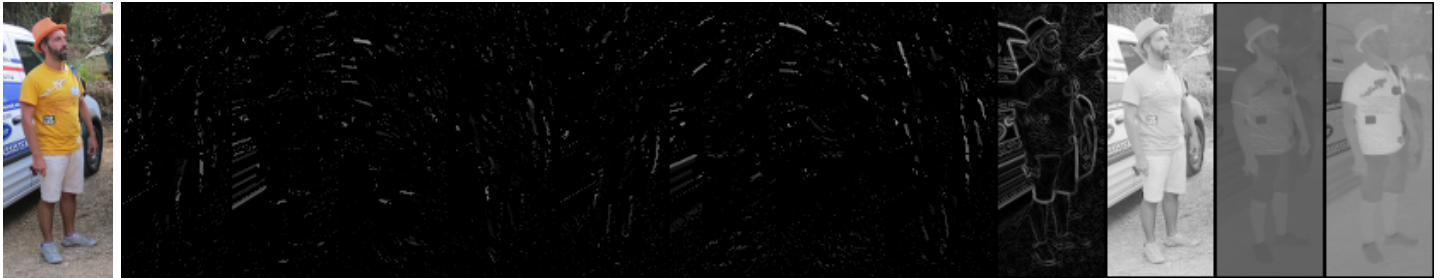
Figure 6.3: Image of the channels used by ICF. From left, the original image is followed by images of the different channels: 8 channels for the quantized gradient phase, 1 channel for the gradient magnitude, and 3 channels for the LUV components, respectively.
