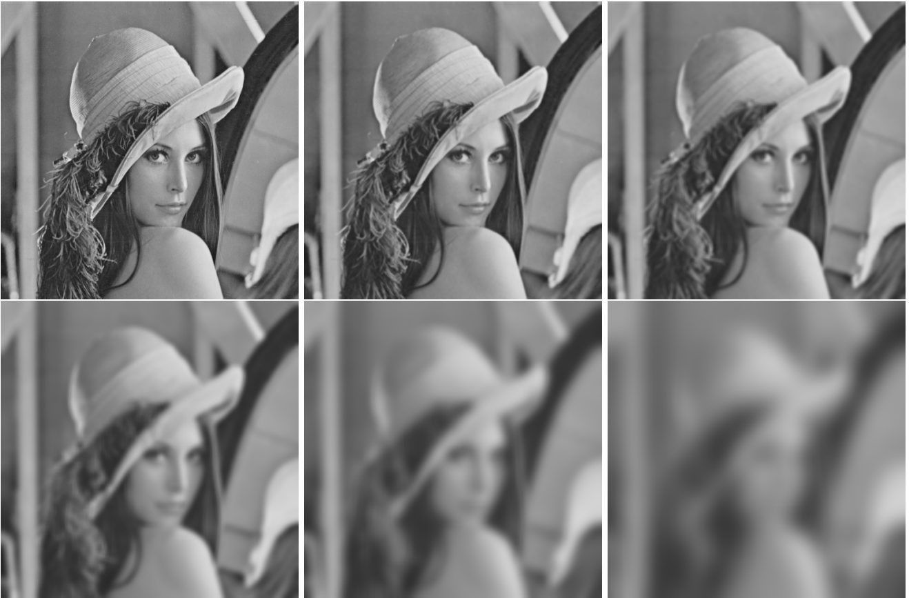
Figure 5.2: Scale-space representation of an image 512 \times 512 : from the original image t = 0 to scales 1, 4, 16, 64, and 256.
