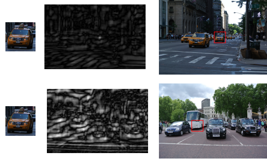
Figure 4.1: Example of Template Matching . The approach works well on the source image, but it cannot be extended to other images, especially with significant variations in brightness and scale.
