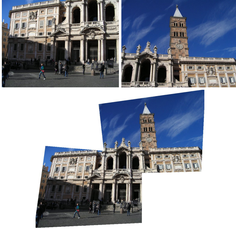
Figure 1.7: Example of homographic transformation: the homography relates 'virtual' planes to each other.
