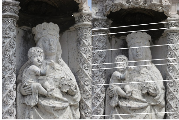
Figure 9.3: The Fundamental matrix allows for the identification of epipolar lines, shown in the right image, on which the corresponding points of the left image reside.
