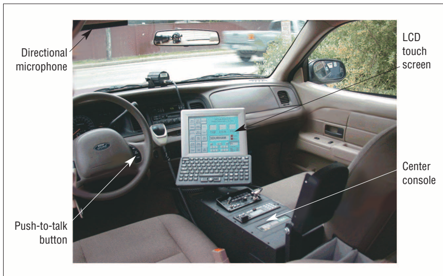
Figure 3. Project54 system hardware installed in a New Hampshire State Police cruiser.
