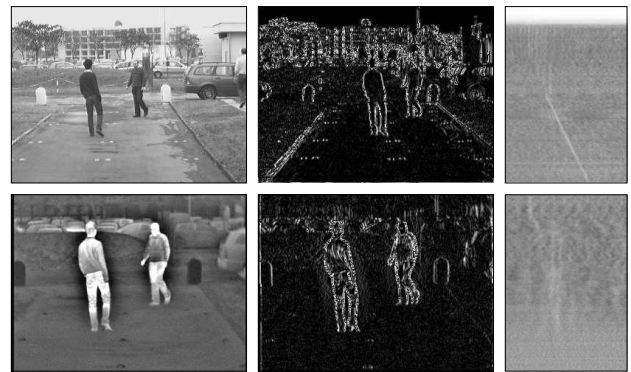
Fig. 1. V-disparity computation in visible and infra-red domains: (left) original images, (center) Sobel images, and (right) correlation map.
