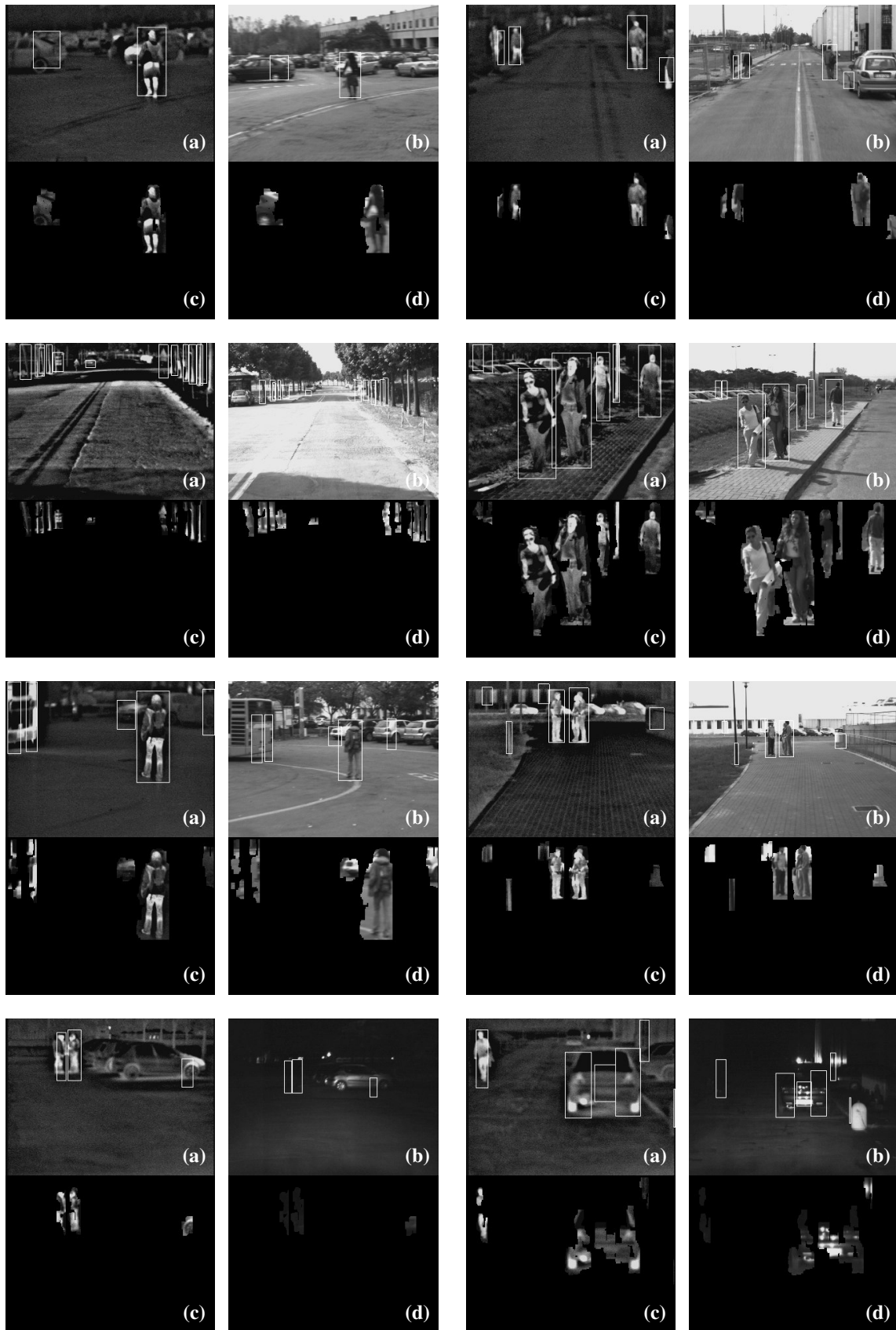
Fig. 8. Few results in different situations: with few or many obstacles, simple or complex situations, day or night time. Images (a) and (b) show the resulting list of bounding boxes superimposed onto the original far infra-red and visible images respectively, and (c) and (d) present the detected obstacles without the background. It can be noticed that the system is able to detect obstacles even when one of the two stereo systems fails the detection.
