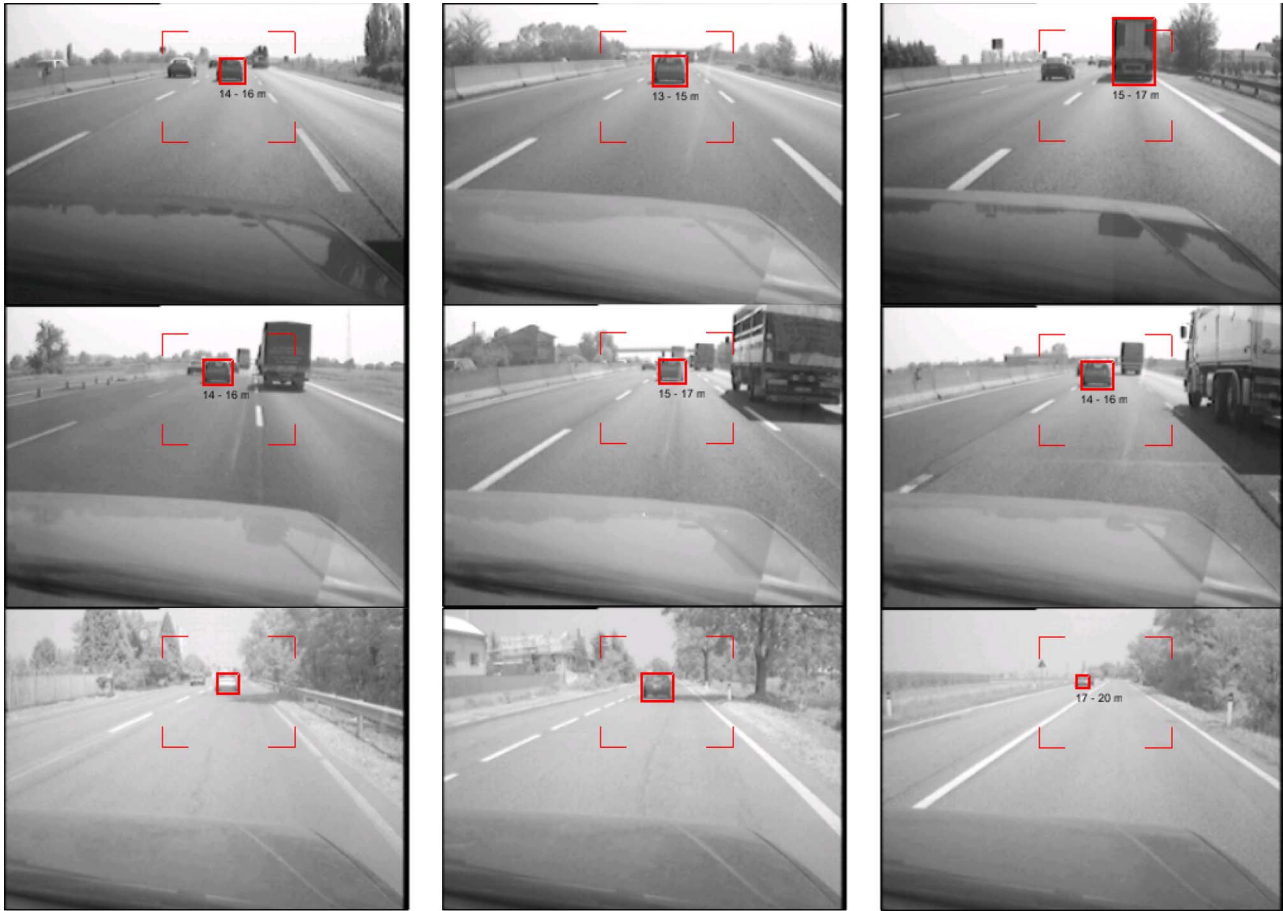
Fig. 13. Results of the preceding vehicle detection in different situations, the detected vehicle is shown using a red bounding box superimposed onto the original image. The four red corners indicate the area of interest when no vehicle is being tracked; anyway, when in tracking mode, vehicles can be detected outside this area. As shown, even vehicles coming toward the vision system are detected as well. The range distance of the vehicle is shown below the red box. If the number of the 3-D points of the detected vehicle is below a predefined threshold, then its distance is not computed. (Color version available online at http://ieeexplore.ieee.org .)
