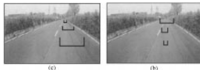
Fig. 13. Detection of the lower part of the bounding box. (a) Correct position and size, taking into consideration perspective constraints and knowledge on the acquisition system setup, as well as typical vehicles' (b) Incorrect bounding boxes.
