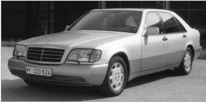
Figure 1. Vamp prototype. Universität der Bundeswehr developed Vamp in 1995 with an automatic trip from Munich, Germany, to Odense, Denmark.
