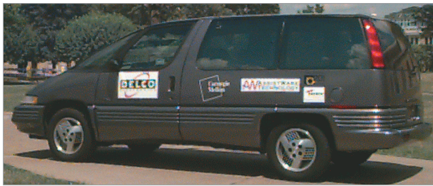
Figure 2. NavLab prototype. Developed by Carnegie Mellon University, NavLab traveled in automatic mode across the US in 1995.
