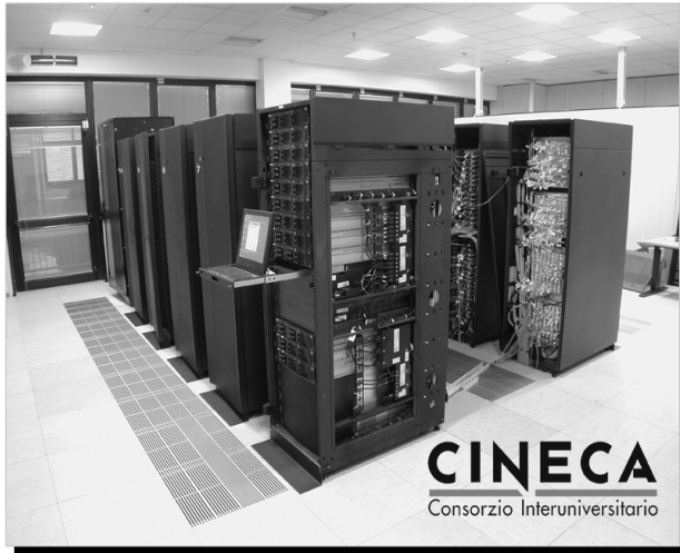
IBM LINUX CLUSTER 256 x 2 Intel Xeon 3 GHz 524 Gbytes RAM 5,5 TB disco
