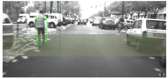
Fig. 6. The pedestrian detection algorithm and filtering provided by motion stereo. Boxes are proved by pedestrian detection algorithm, light green boxes are definitely detected, dark green boxes are the rejected by motion stereo
