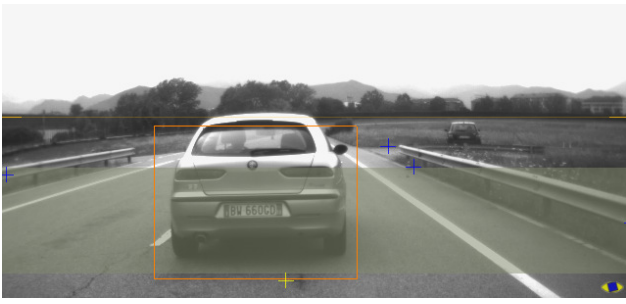
Fig. 5. Vehicle detection using radar and vision fusion: the orange box contains the final result of vehicle detection, the yellow cross is the refined radar beam associated to vehicle and the blue crosses correspond to discarded beams.
