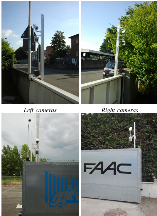
Fig. 3. Real environment gates setup: sliding gate (above) and swing gate (below) with a NIR illuminator installed below each camera.
