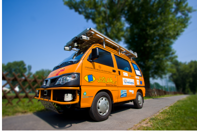
Fig. 5. Autonomous Piaggio Porter. It mounts several stereo vision systems, with different baselines, that look in different directions. It also has four laser scanner that cover the area all around the vehicle
