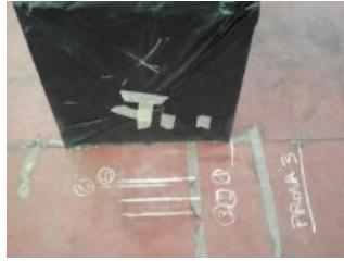
Fig. 11. Example of dark cube used in breaking tests. The white lines on the floor representing the LGV stop positions in different tests.
