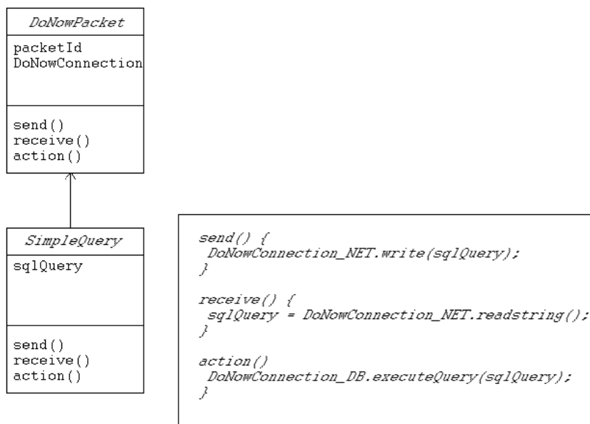
Fig. 3. Example of a simple packet implementation.
