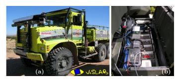
**Fig. 2.** The TerraMax vehicle (a) and its on-board PCs (b) fitted under the passengers seat.
