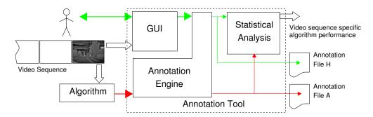
Fig. 1. Block diagram of the algorithm: human and algorithm process the same video sequence producing annotation files H and A. The two files are compared producing statistics about algorithm performance
