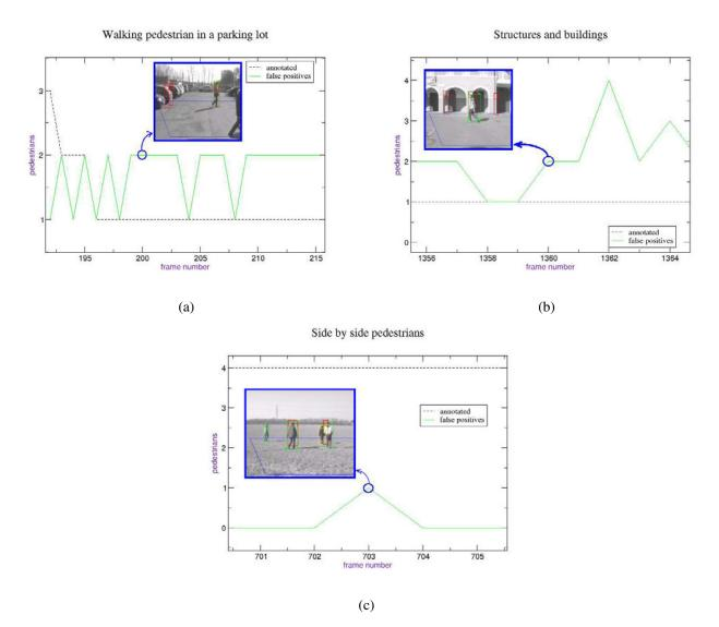
Fig. 4. Examples of situations in which the human shape detection algorithms partially fails: (a) background noise generated by parked vehicles introduces false positives; (b) columns generate false positives due to their symmetry; (c) two pedestrians walking side by side mislead symmetry evaluation.
