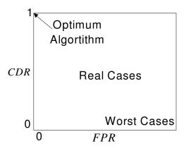
Fig. 3. Vision based pedestrian detection normalized evaluation space.
