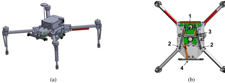
Fig. 1: Proposed system setup consists in an enhanced DJI consumer drone. (1a) Perspective view of the modified DJI Matrice 100. (1b) Bottom view with highlighted perception suite: (1) custom processing board; (2) lateral stereo pairs; (3) down-looking stereo pair; (4) front-looking stereo pair.
