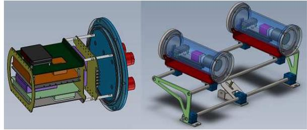
Fig. 2. 3D CAD model of the vision system: vision canister (left) and stereo rig (right).
