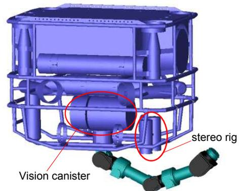
Fig. 1. 3D CAD model of the MARIS AUV. The horizontal stereo rig points to the bottom of the vehicle.
