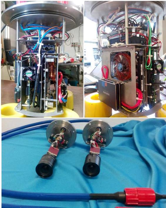
Fig. 4. Components of the vision system: internal view of the vision canister (top images); AVT Mako cameras, optics and cabling (bottom image).
