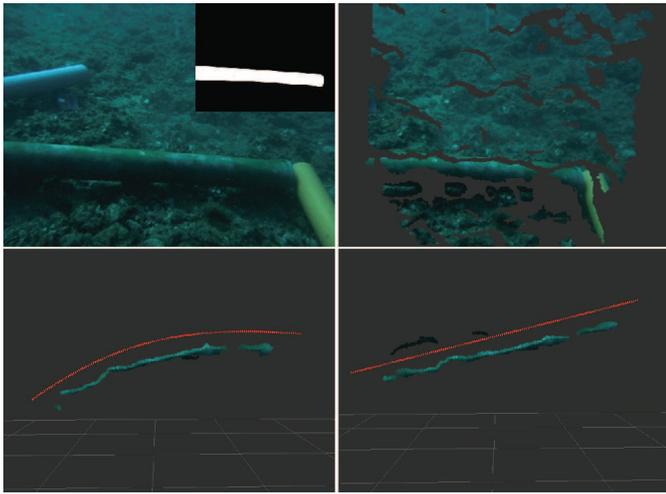
Fig. 6. Example of the automatic calibration approach. Left camera image and segmented pipe (top left). 3D point cloud from disparity map (top right). Distorted pipe using in-air calibration parameters (bottom left). Pipe rectification using optimized camera parameters (bottom right). Red dotted line is displayed to ease the graphical interpretation.
