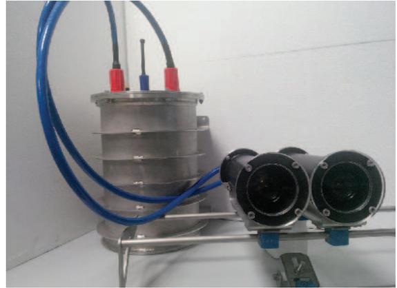
Fig. 3. Underwater vision system: vision canister (left) and the stereo rig (right) with the two camera canisters.
