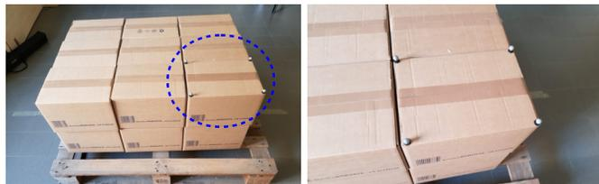
Fig. 6. Configuration *A*, with four OptiTrack markers temporarily placed on the box in the lower right corner, highlighted by a blue circle (left). Close-up detail of the box (right).
