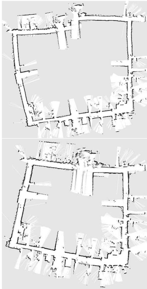
Figure 2: Map of the environment of dataset ACES before (top) and after (bottom) a loop closure is solved with the proposed algorithm.
