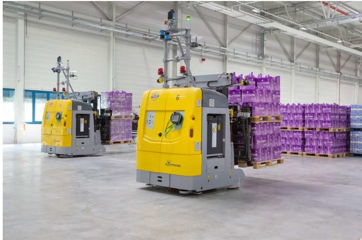
Figure 1: An industrial AGV (Elettric80 CB25) equipped with a navigation laser scanner at the top of a telescopic pole.
