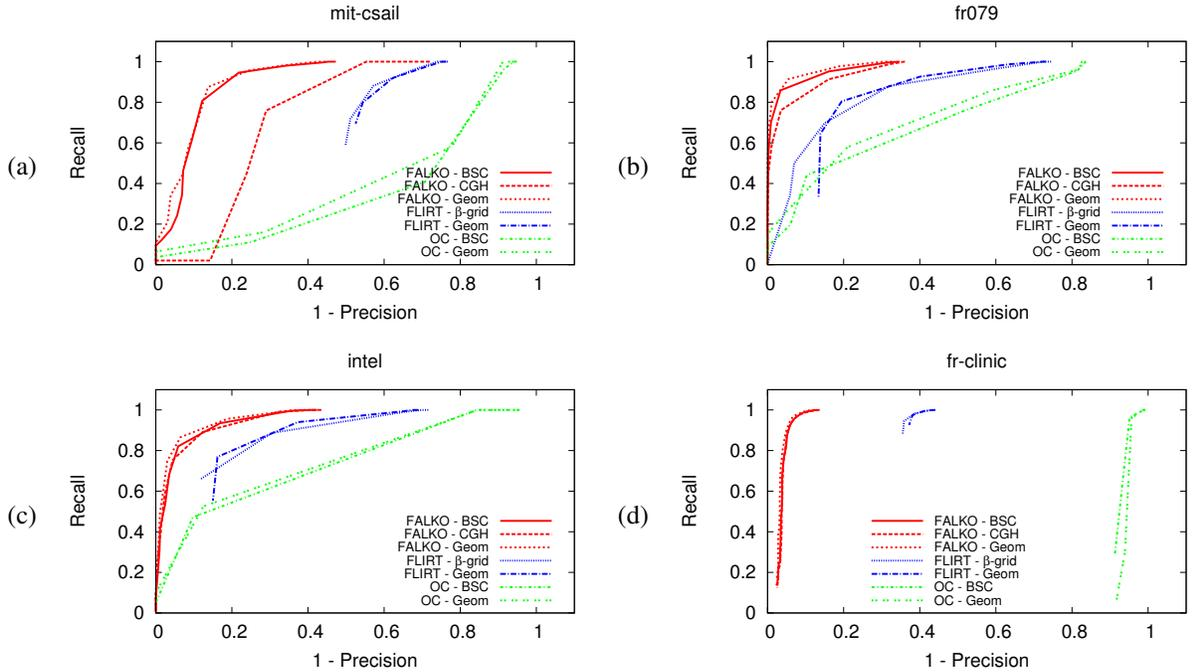
Fig. 6: 1-Precision Recall curves of global localization with FALKO- $\{\text{BSC, CGH, Geom}\}$ , FLIRT- $\{\beta\text{-grid, Geom}\}$  and OC- $\{\text{BSC, Geom}\}$  for datasets (a) mit-csail, (b) fr079, (c) intel, and (d) fr-clinic.
