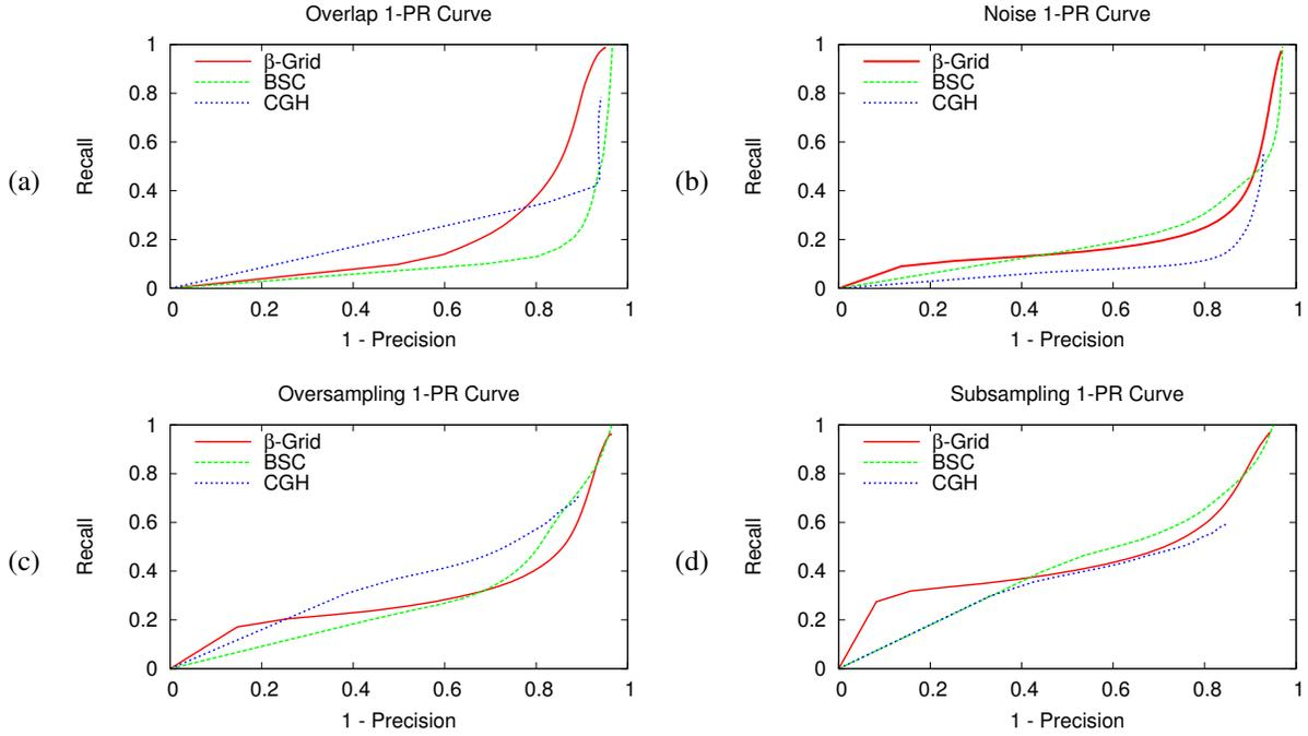
Fig. 5: 1-Precision Recall curves for the descriptors  $\beta$ -grid, BSC and CGH in four tests: (a) viewpoint (scan overlap value in interval 50% – 90%); (b) noise level; (c) oversampling of scan measurements; (d) subsampling of scan measurements.
