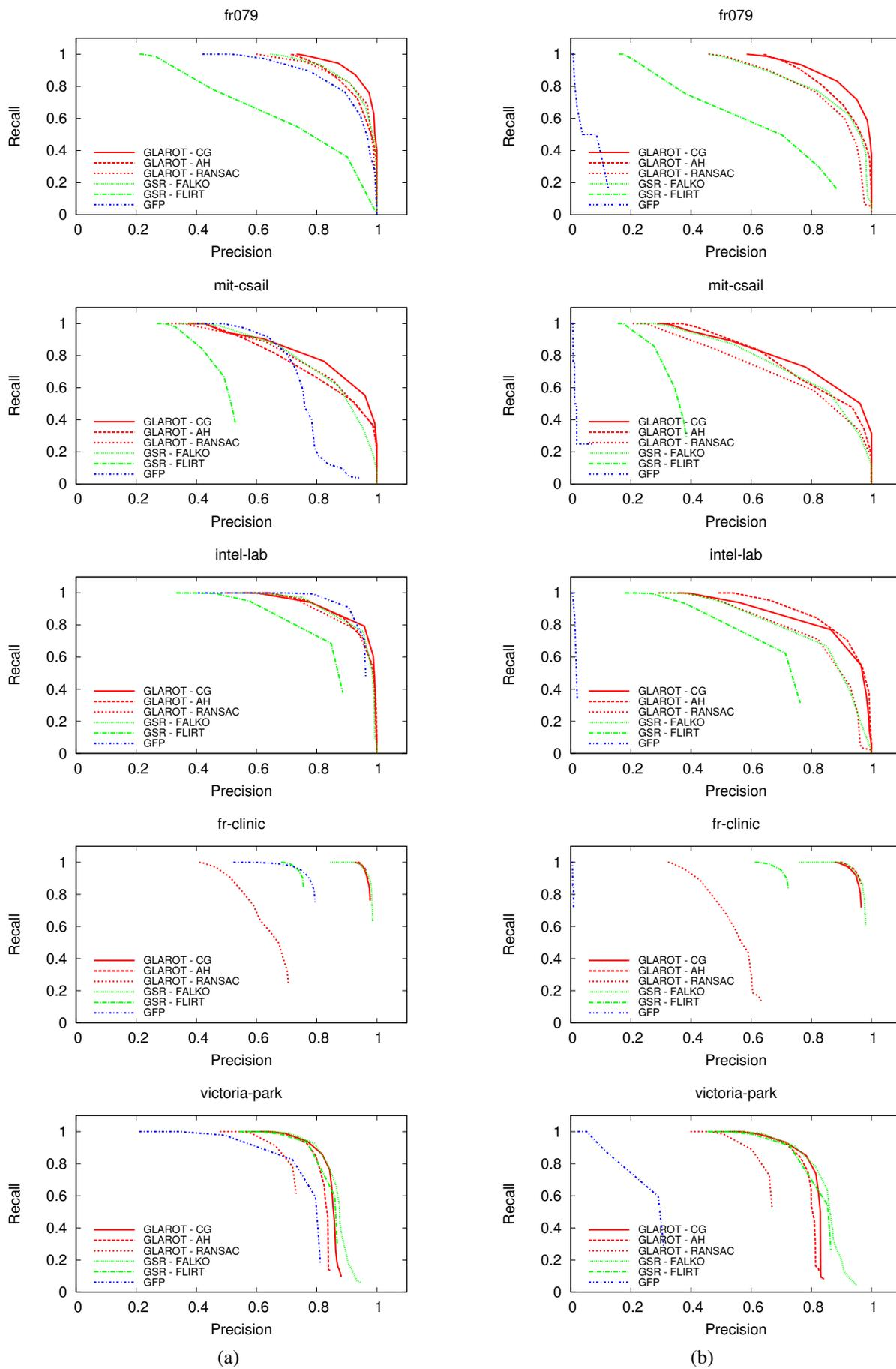
Fig. 3: Precision-Recall curves for offline (a) and online (b) loop-closure tests.
