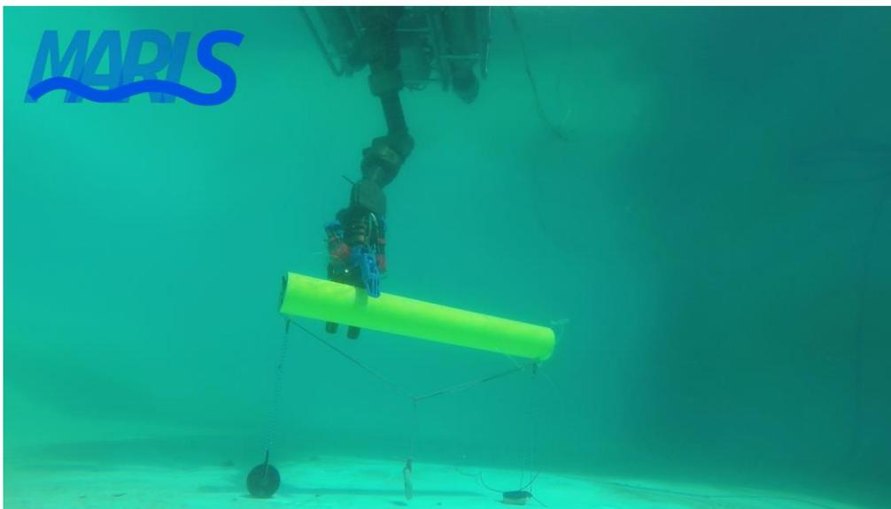
Fig. 4: Underwater view of single-agent experimental grasp operation
