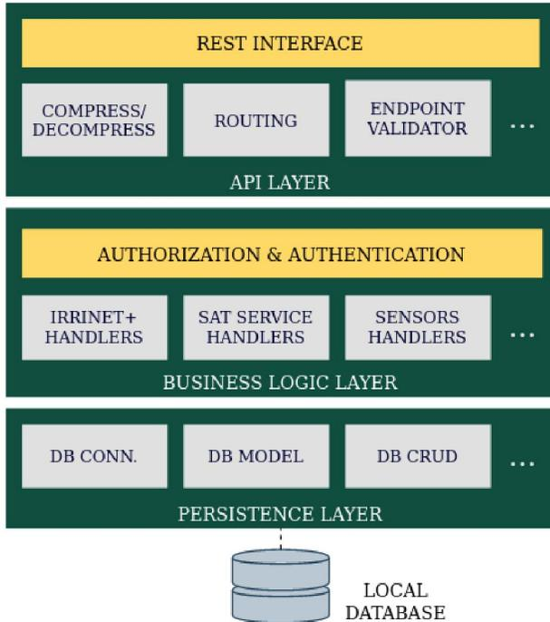
Fig. 2. Logical structure of the POSITIVE Server.
