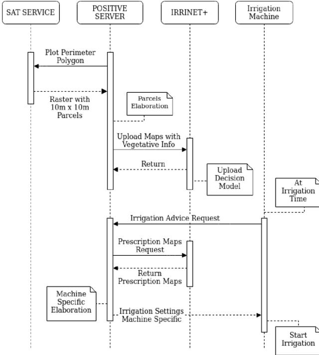
Fig. 3. Sequence Diagram of the data flow producing a machine-specific irrigation recipe.
