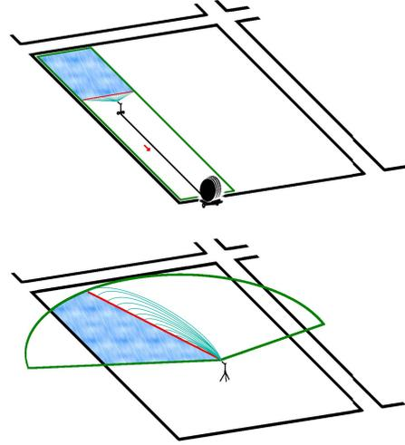
Fig. 4. Schema illustrating the linear (top) and central pivot (bottom) irrigation machines and the respective partition of the fields into strips and angular sectors.
