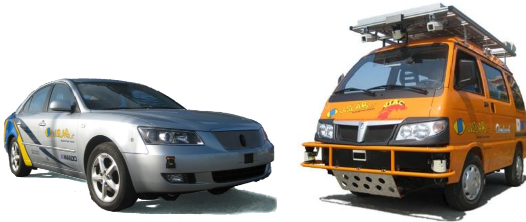
Figure 5: Different integration levels on two prototypes of autonomous vehicles developed by VisLab: BRAiVE and the vehicles used for VIAC
