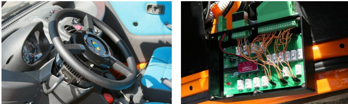
Figure 12: left: the TopCon steering system and the board to control gas
