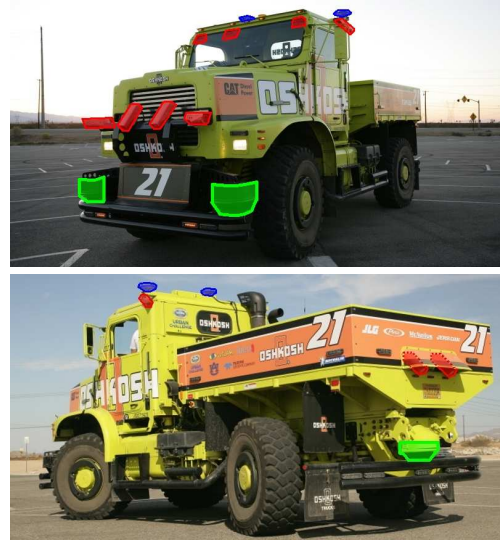
Fig. 3. All the Terramax sensors highlighted. Color coding: red – cameras; green – LIDARs; blue – GPS antennas.
