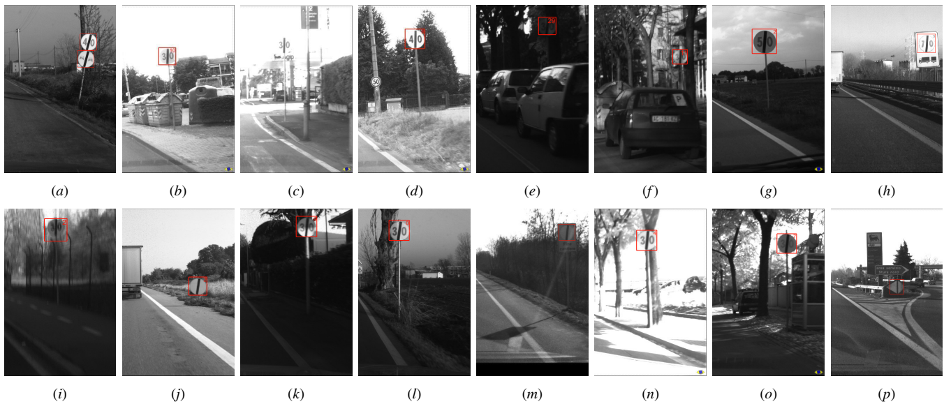
Fig. 13. De-restriction sign detection (although the algorithm processes the whole image, only the right half of the image is showed for space reasons): (a) detection of two de-restriction signs in the same image; (b) with light contrast between the sign and the background; (c) without contrast between the sign and the background, the sign can not be detected; (d) in a rolled image, in presence of partially saturate background; (e) in a dark image; (f) spot shadows; (g)-(h) end of 50 and 70 km/h speed limit; (i) in a blurred image; (j) sign placed on the ground; (k) top and bottom of the sign differently enlightened; (l) right and left sides of the sign differently enlightened; (m) smaller, inside a square panel; (n) partially saturated background; (n)-(o) with trees; (p) false positive.
