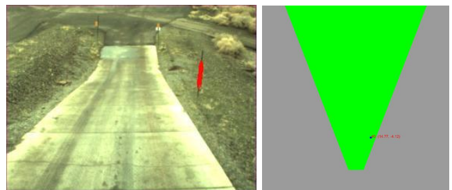
Fig. 10. Obstacles bird's eye view map for example of Fig. 9. The field of view is shown in green.
