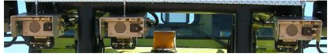
Fig. 2. TerraMax camera setup. The three cameras feature a 640 \times 480 -pixel Bayer-pattern output and mount low distortion 6-mm optics. Synchronization is directly supplied by the cameras through the firewire bus.
