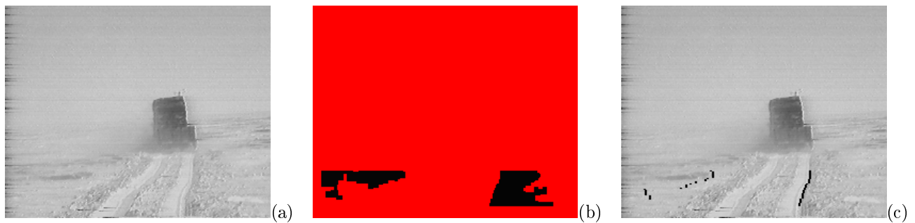
Figure 15. An example of wrong detection due to a non correct camera orientation: (a) input image, (b) connected areas, (c) high level analysis result.
