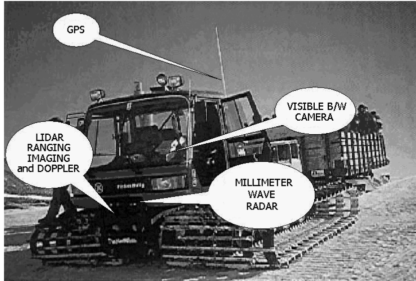
Figure 1. Photo of the snowcat and its sensing capabilities.
