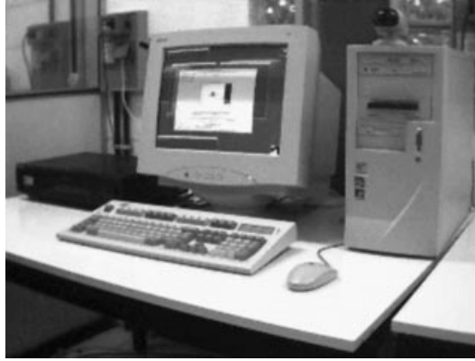
Figure 2. The current system: on the left it is visible the video recorder used to acquire data; the video camera that produces the composite signal for the real-time acquisition is also visible on the top right side.
