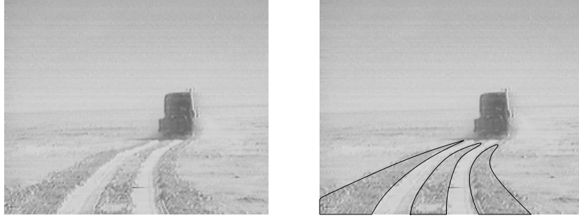
Figure 6. Original image and dark areas that represent the interesting regions whose precise position needs to be extracted.
