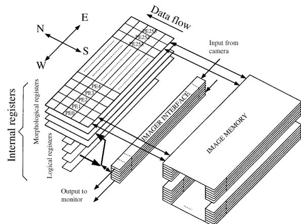
Figure 5. Structure of a 256 PEs Processor Array.
