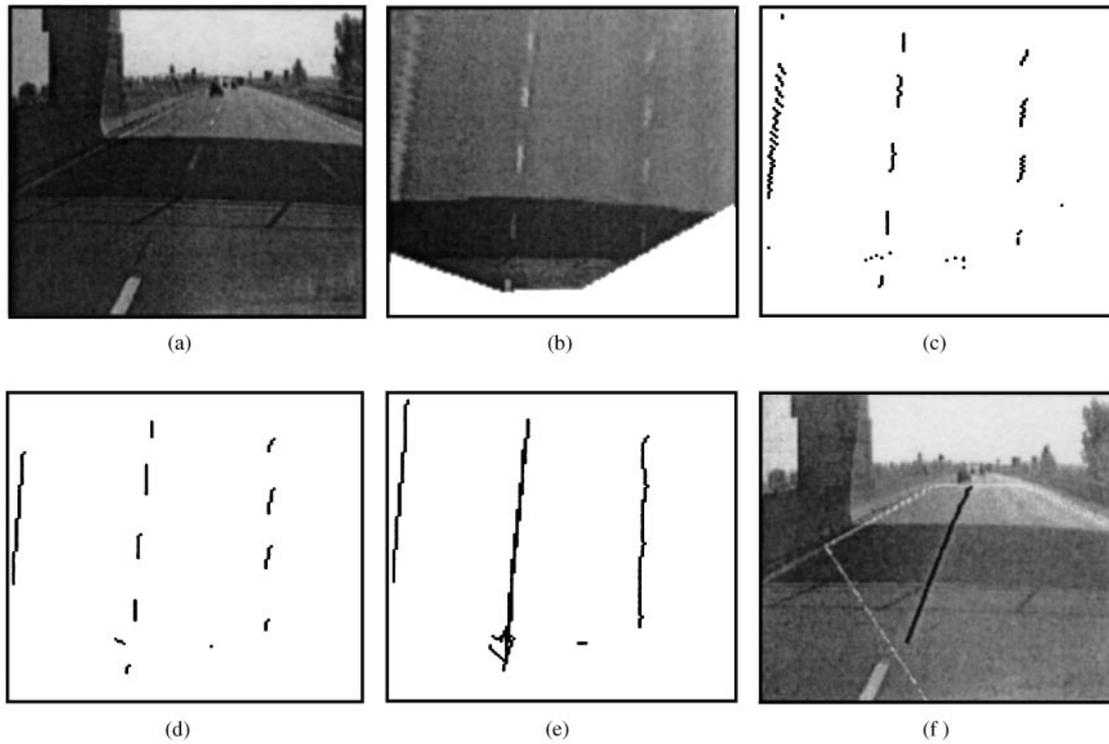
**Figure 3.** Lane Detection steps: (a) the captured image; (b) after the removal of the perspective effect; (c) pixels with darker horizontal neighbors; (d) chains of non-zero pixels; (e) the joined polylines; and (f) the computed center line superimposed in black onto a brighter version of the acquired image.
