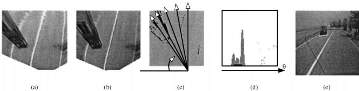
**Figure 4.** Obstacle Detection steps: (a) the left remapped image; (b) the right remapped image; (c) the difference image and the angles of view; (d) the polar histogram; (e) the obstacle detected shown by a white marker superimposed onto a brighter version of the left acquired image.
