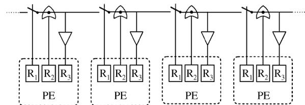
**Figure 6.** Interprocessor Communication Network (ICN): for each PE, Register  $R_1$  drives its ICN switch; Register  $R_2$  sends its value over the network; and Register  $R_3$  collects the resulting value from the network.
