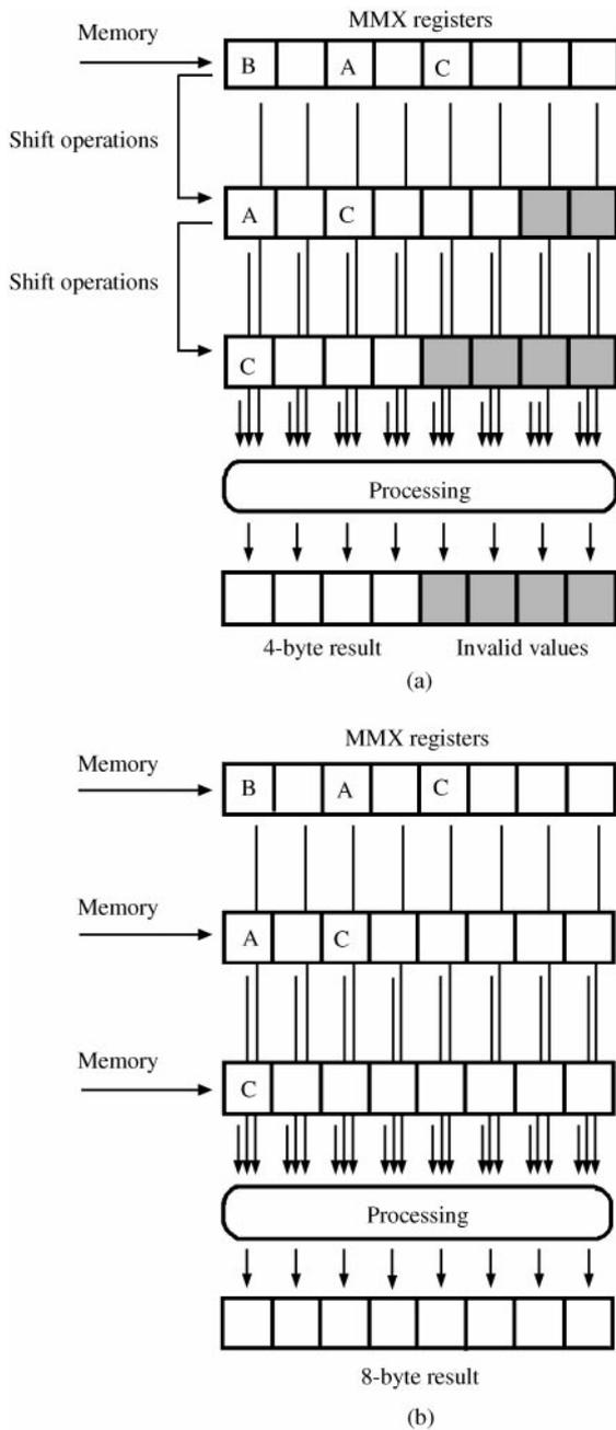
**Figure 8.** Two different approaches to a cellular automation operation in the MMX technology involving 8-bit pixels A, B, and C: (a) a single access to the memory followed by shift operations; (b) three partially overlapped accesses to memory.
