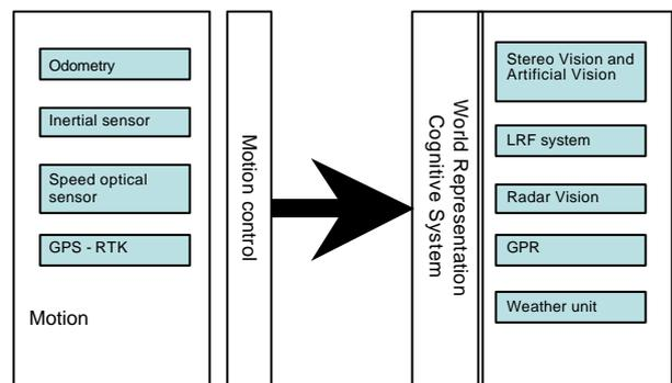
Fig. 1 – simplified sensing architecture of RAS
