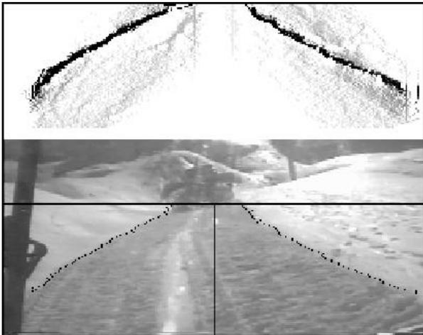
Fig. 6 – Examples of the best path selected by the ants; the upper part of each image encodes the number of ants passed on each pixel.
