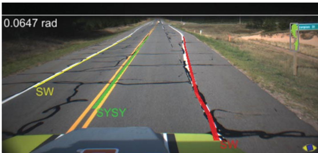
Figure 6. Results of lane detection algorithm projected on the original image. From right to left, the red line represents a right boundary, green a left boundary, and yellow a far left boundary. In this image, the right line is detected although it is not a complete line.
