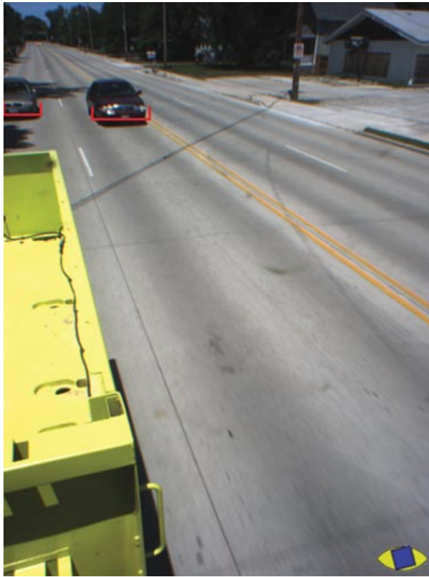
Figure 9. Rearview system algorithm results (detected vehicles are marked in red).
