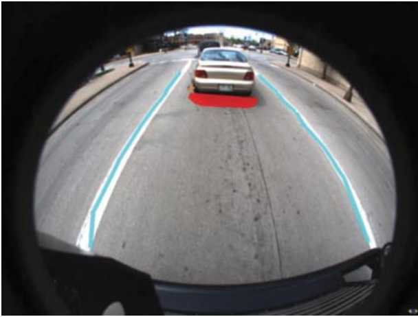
Figure 7. A sample frame showing typical obstacle and lane detection.
