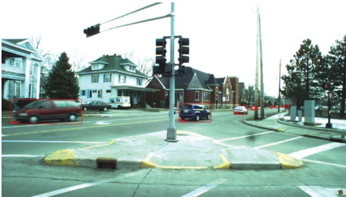
Figure 8. Lateral system algorithm results (detected vehicles are marked red).
