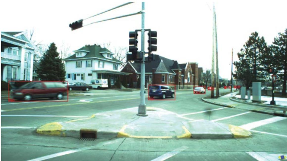
**Figure 8.** Lateral system algorithm results (detected vehicles are marked red).
