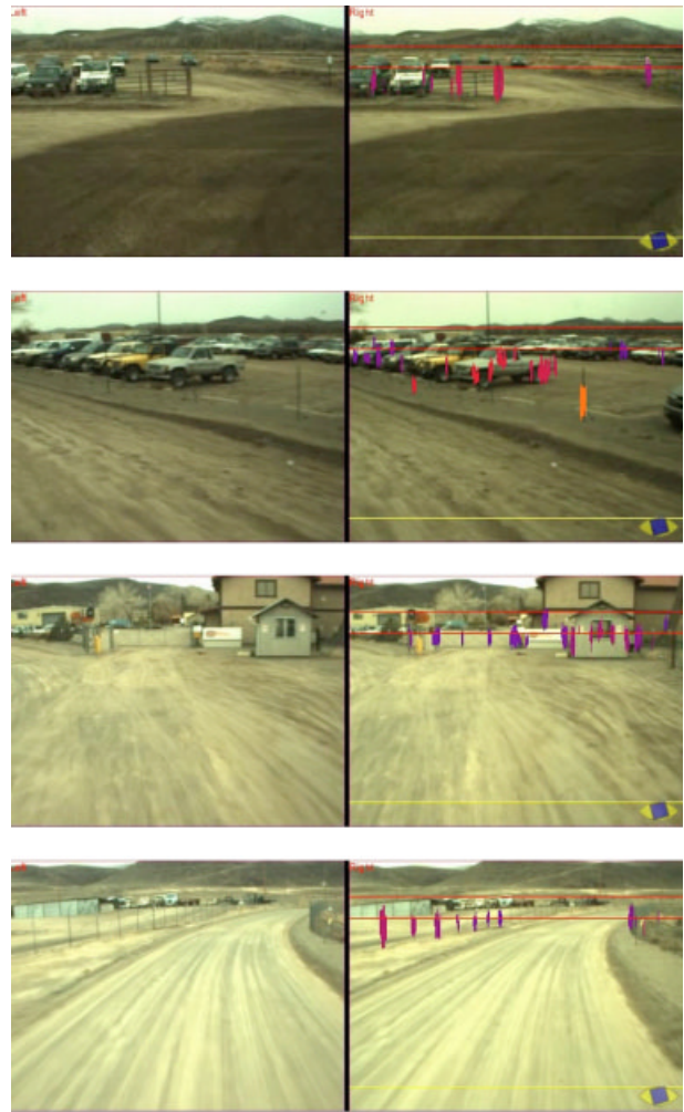
Figure 14. Images showing left and right images of different situations; on the right images, colors show the presence of detected obstacles: different colors mean different distances. The additional horizontal lines represent the 5 m, 50 m, and horizon position. Posts and thin poles are correctly detected.
