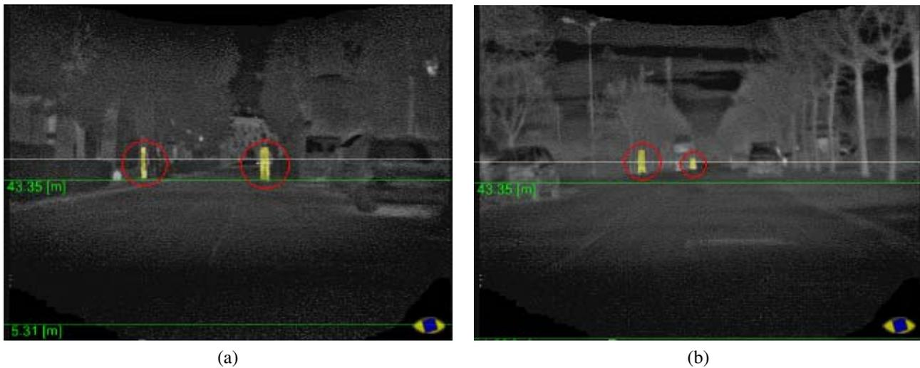
Fig. 9. In (a) a cyclist is recognized as a pedestrian, together with a standing person. In (b) an example of misdetection: the hot spot on the right is a vehicle light.
