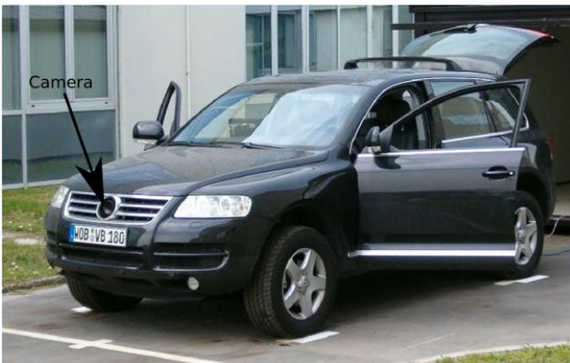
Fig. 4. Vehicle equipped with a FIR camera used for testing the algorithm.
