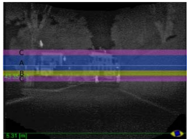
Fig. 5. Image acquired when driving on a speed bumper. The heavy calibration error causes the pedestrian to appear inside region C, so that it cannot be recognized.
