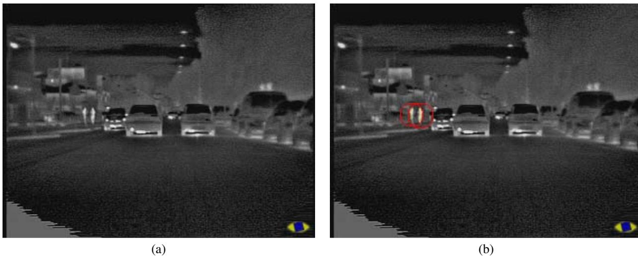
Fig. 6. An example of algorithm output: in the original image (a) two distant pedestrians are present; they are both recognized by the algorithm (b).
