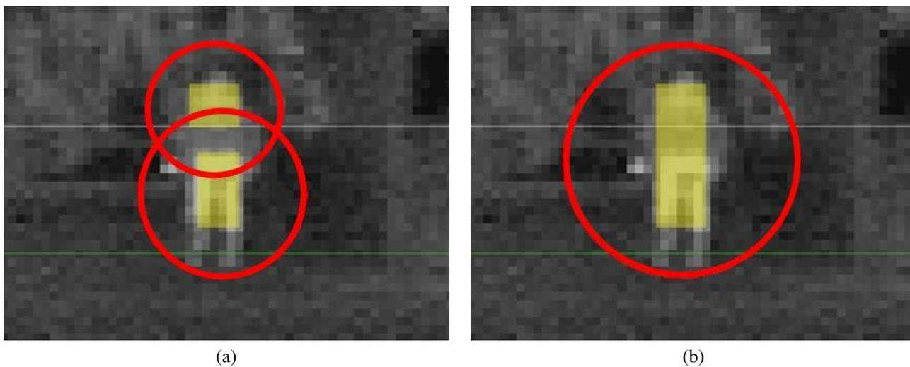
Fig. 8. In (a), a pedestrian is recognized as two separate hot spots, due to the cold trunk; the merging phase can solve this problem by creating a single, larger hot spot (b) that can be recognized as a pedestrian in the following validation step.
