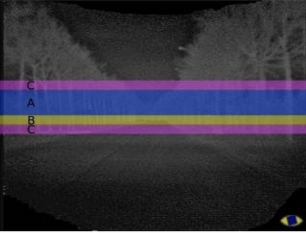
Fig. 2. Detection regions. A bounding box containing a distant pedestrian should be inside areas A and B. Bounding boxes overlapping also on C are discarded.
