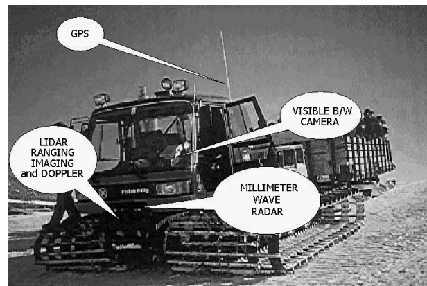
Fig. 1. The snowcat and its sensing capabilities.
