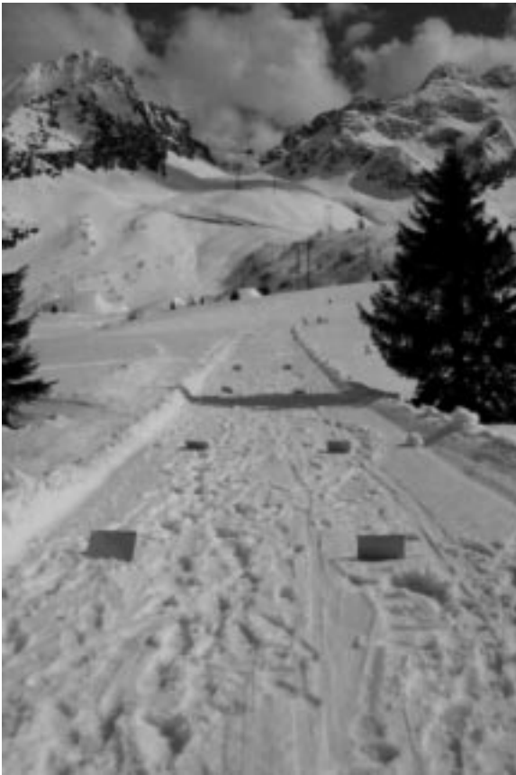
Fig. 8. Image of the test site on the Italian Alps; a patch of snow with markers is used to calibrate the cameras.
