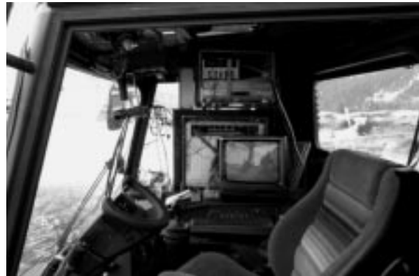
Fig. 6. Inside view of the vehicle during a test; the stereo cameras are visible on the left-hand side.
