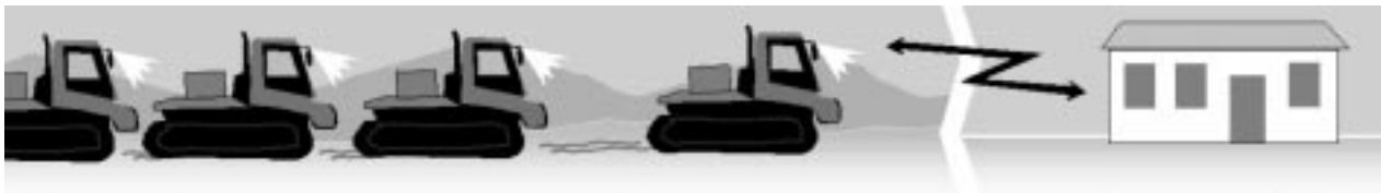
Fig. 3. Platoon of snowcat vehicles; the first will be either manually driven by an expert driver or remotely driven from the Italian base; all the others will follow automatically, using visual information only.
