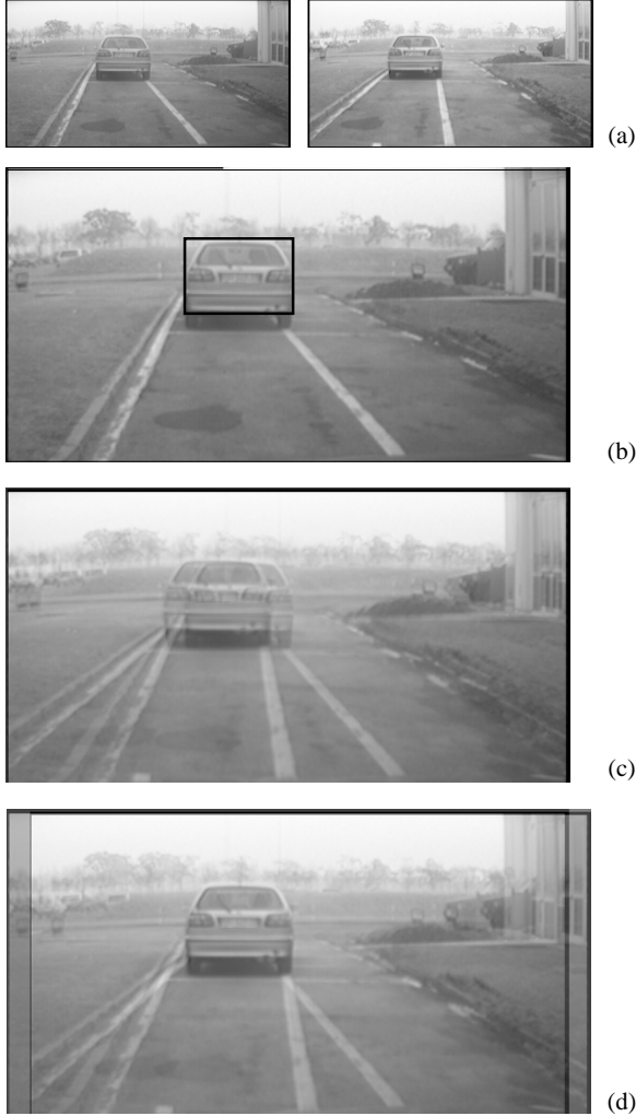
Figure 10: Distance refinement: (a) left and right stereo images; (b) incorrect result of the detection step (the lower part of the bounding box indicates a wrong distance); (c) superimposition of stereo images with a null offset; (d) superimposition of correctly shifted stereo images.
