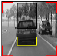
Figure 8: The search area for the upper part of the bounding box is shown in dark gray. It takes into account knowledge about the typical vehicles' aspect ratio.
