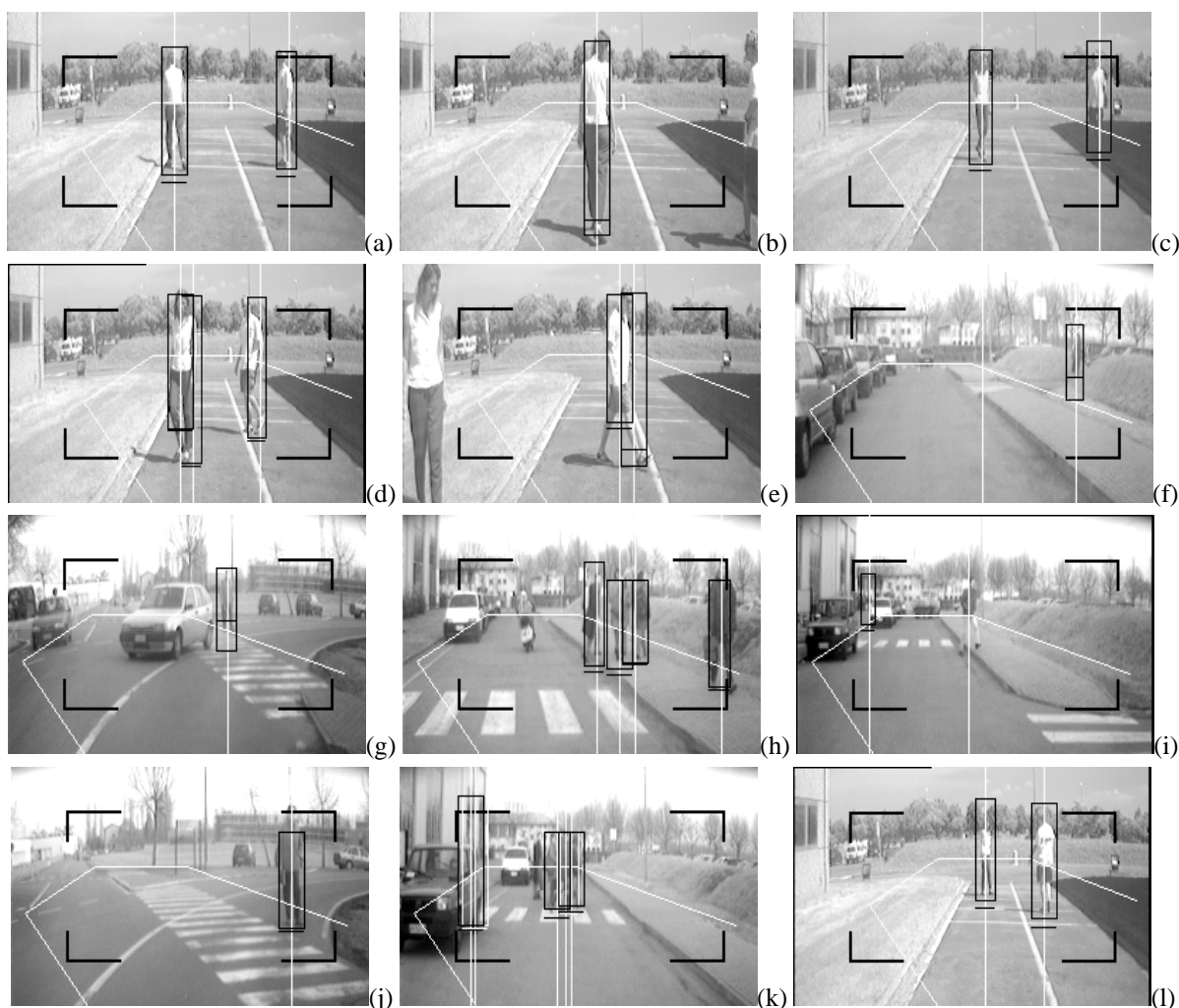
Figure 10: Pedestrian detection results: images show the symmetry search area (delimited by black corners) and the detected pedestrians, each with the symmetry axis (in white) and bounding box (in black). The horizontal black segment shows the distance obtained from the monocular analysis, prior to stereo refinement. The trapezoidal white line delimits the road surface portion visible by both cameras.
