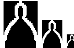
Figure 8: Binary model used to localize the pedestrian's head: different sizes are considered.
