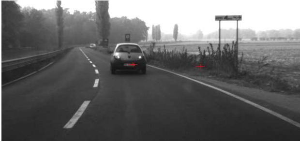
Fig. 1. Camera miscalibration caused by pitch variation: the radar point is not correctly represented on the vehicle base
