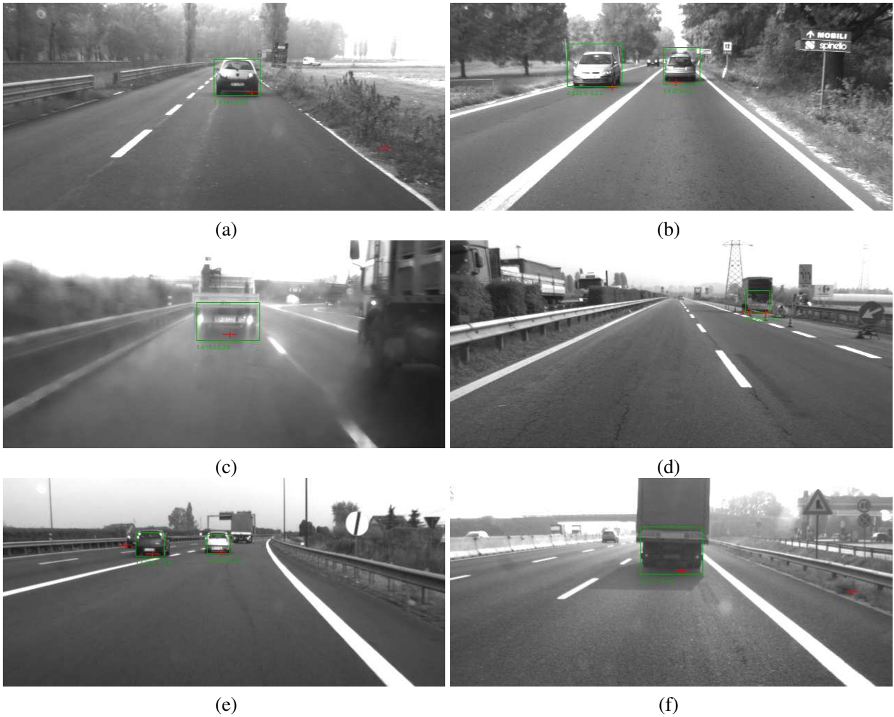
Fig. 7. Examples of correct results: the algorithm works reliably in simple cases (a); it detects both vehicles moving away and approaching (b); it works even in hard cases, such as rain (c) and noisy scenario (note the double radar detection) (d); it can detect cars (e) and truck (f).
