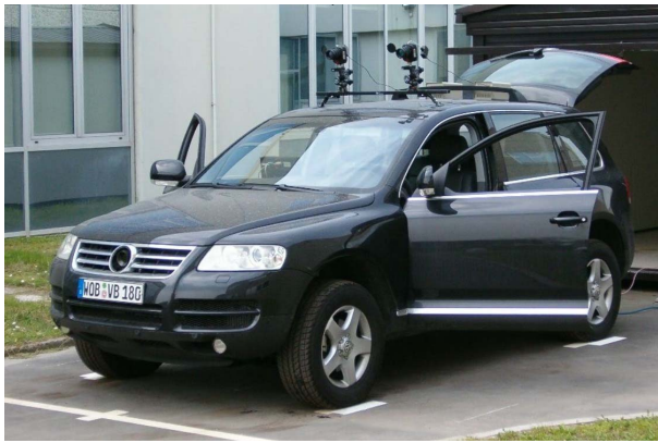
Fig. 1. The test vehicle with different camera mounting examples: front camera above the license plate and two cameras on the top of the vehicle.
