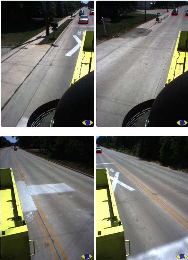
Figure 8. Some results of the RearView system. When a car is in the lane at the back of the truck, it is shown with a red marker.
