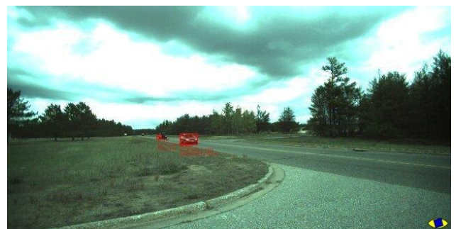
Figure 9. Result of the Lateral system: incoming vehicle are detected at crossroads.
