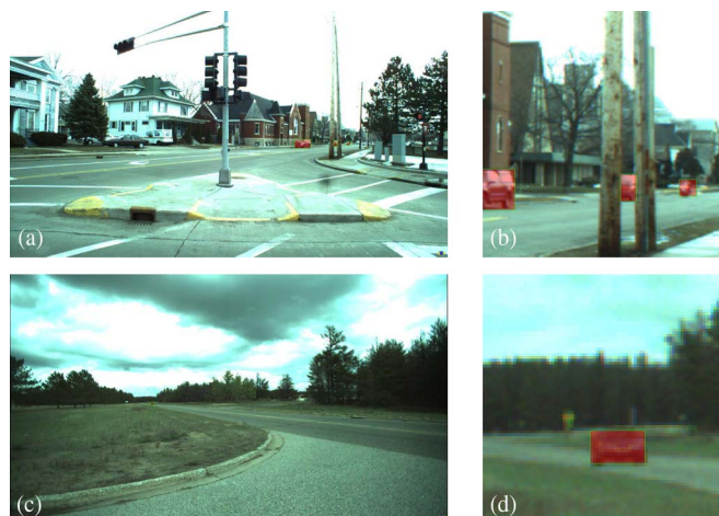
Fig. 16. Detection results. The left column shows the complete result images, and the right column shows the same images zoomed in to highlight far-away detected objects.
