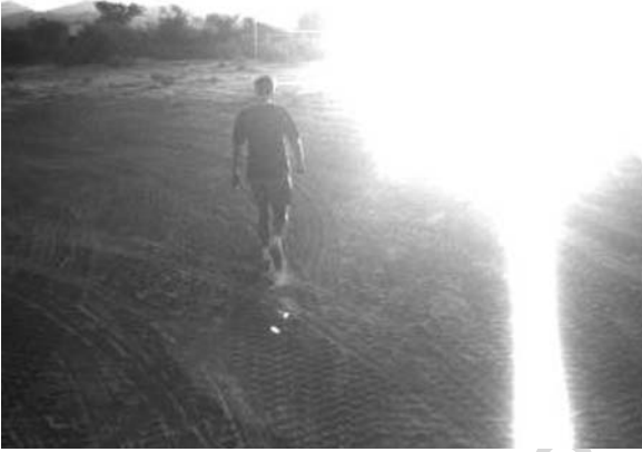
15 Fig. 18.9 Example of automatic exposure control obtained by defining a specific area (matched 16 with the application) in which the contrast and brightness should assume optimal values
