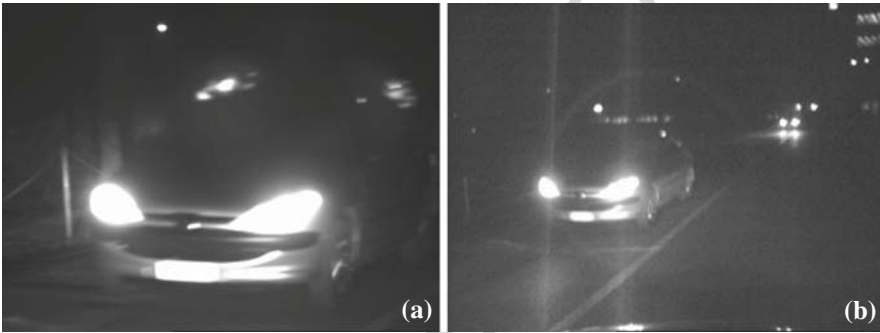
29 Fig. 18.10 Smear effect in (a) visible cameras and (b) NIR devices
