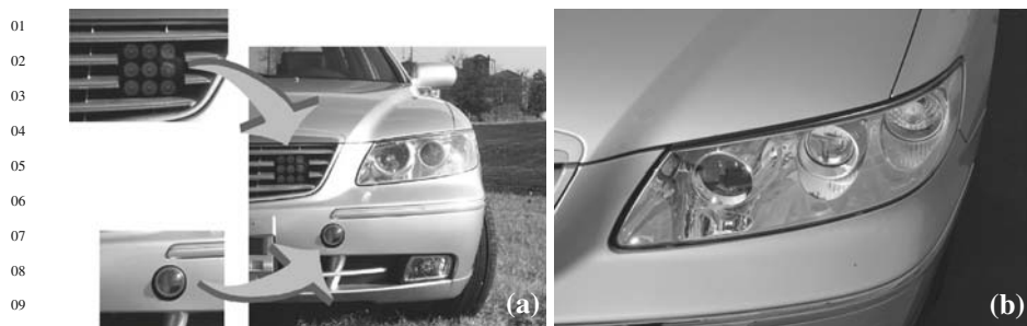
Fig. 18.5 Two different types of near-infrared lamps installed on an experimental vehicle (a). Night vision lighting system composed by low/high beam light to the left , NIR lamp in the middle , and parking light to the right (b)
