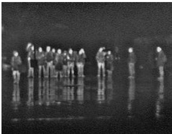
Fig. 18.11 Reflection of a wet surface for far-infrared radiations
