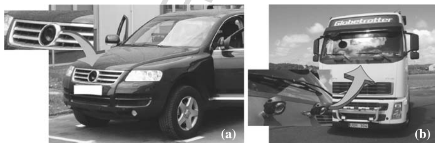
Fig. 18.3 Example of integrating of a FIR vision system: an infrared camera is mounted in a central position in the front of the vehicle (a). Integration of a stereo vision system on a truck (b)
