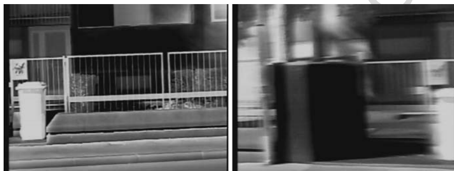
Fig. 18.8 An example of motion blur in FIR images acquired by an onboard vision system: the left image was captured when the vehicle was still, while the right photograph was taken only a few seconds later – when the vehicle turned left – and shows a heavy horizontal motion blur effect
