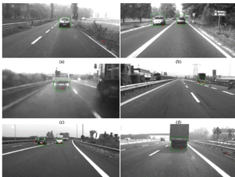
Fig. 1. Examples of correct results: the algorithm works reliably in simple cases (a); it detects both vehicles moving away and approaching (b); it works even in hard cases, such as rain (c) and noisy scenarios (note the double radar detection) (d); it can detect multiple cars (e) and truck (f).
