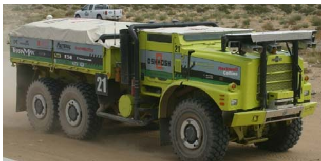
Figure 1: Oshkosh Truck unmanned vehicles: TerraMax™, based on MTRV, (left) and autonomous PLS (right)
