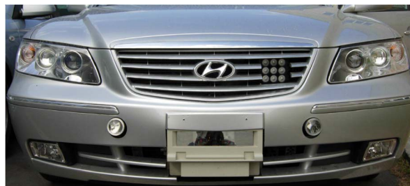
Fig. 5. Detail of the front bumper showing the laser scanner integration and the headlights.
