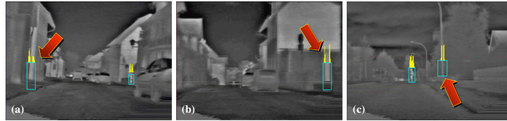
Fig. 5. Filters relying on specific features of artifacts. For each BB the vertical histogram of edges is displayed on top of it. The arrows point discarded BBs.
