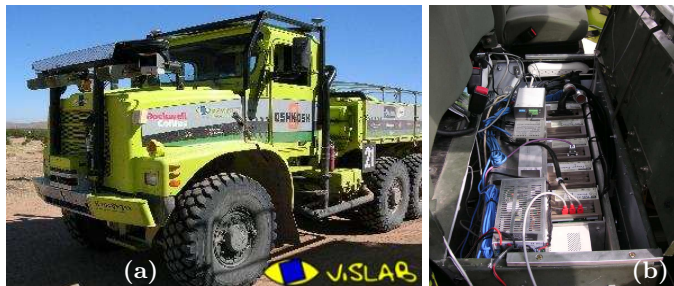
Fig. 2. The TerraMax vehicle (a) and its on-board PCs (b) fitted under the passengers seat.
